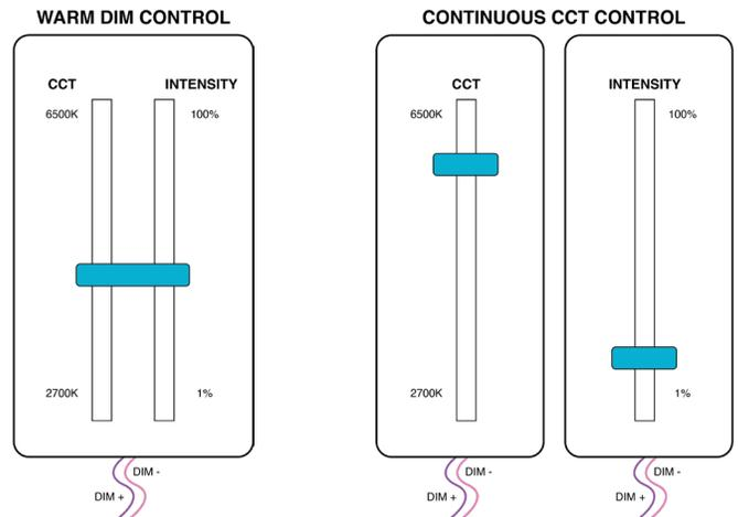
Only one set of dimming Leads are required. As Intensity is Increased so is the CCT. As intensity decreases the CCT decreases to warmer color Temperatures.
